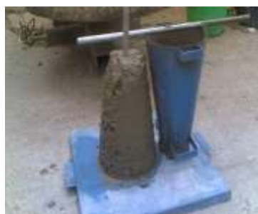
Slump cone test
